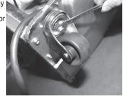
**Note**: Two of the casters include locking mechanisms to ensure the unit does not slide on hard floors. These two locking casters should be fastened at the front end of the unit, with the unlocked casters fasted on the rear end.
